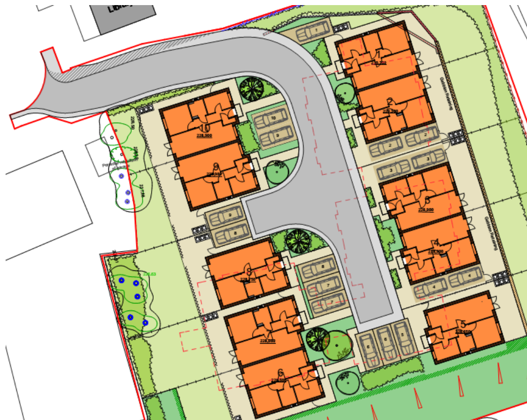
Proposed site access, layout and parking spaces
